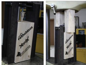
Fig. 2: Test sample and its fixing in hydraulic press – tension parallel to the grain.
