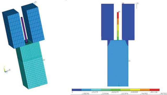
Fig. 3: Finite element network of the tested joint.
