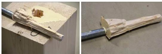
Fig. 4: Tension parallel to the grain – test sample damage
