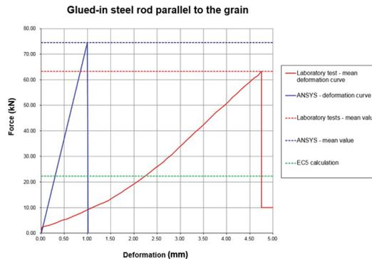
Fig. 7: Glued-in steel rod parallel to grain – results.
