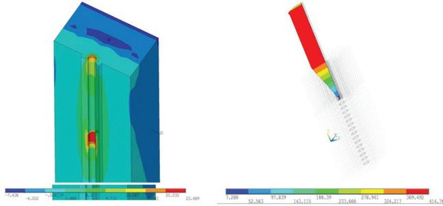
Fig. 5: Tension  $S_x$  and von Mises stress for the force  $F=76.40$  kN.
