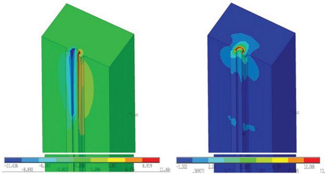
Fig. 6: Shear  $S_{xy}$  and tension  $S_y$  stress for the force  $F=76.40$  kN.
