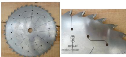
Fig. 4: Circular saw blade 2 with non-uniform tooth spacing and a body with dilatation gaps (Droba and Svoreň 2012).
