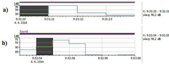
Fig. 11: Graph of the noise course at the cross sectional beech wood cutting: feeding speed  $v_f = 12 \text{ m}\cdot\text{min}^{-1}$ , a) circular saw blade 1, b) circular saw blade 2.
