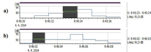
Fig. 5: Graph of the noise course in the cross sectional wood cutting: Feeding speed  $v_f = 4 \text{ m}\cdot\text{min}^{-1}$ , wood species (spruce), a) circular saw blade 1, b) circular saw blade 2.
