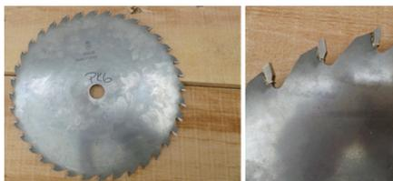
Fig. 3: Circular saw blade 1 with uniform tooth spacing and a full body (Droba and Svoreň 2012).
