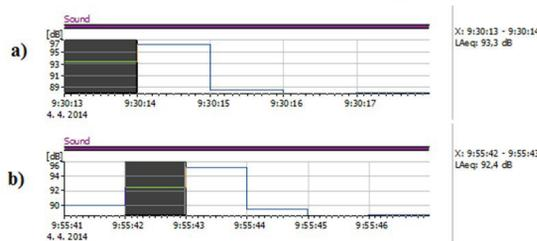
Fig. 10: Graph of the noise course at the cross sectional pine wood cutting: feeding speed  $v_f = 12$  m·min<sup>-1</sup>, a) circular saw blade 1, b) circular saw blade 2.
