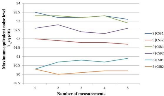
Fig. 12: Comparison of noise level at circular saw blades: feeding speed  $v_f = 12 \text{ m}\cdot\text{min}^{-1}$ , S (spruce), P (pine), B (beech), CSB1 – circular saw blade 1, CSB2 – circular saw blade 2.
