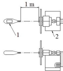
Fig. 2: Scheme for placement of a sound level meter: 1- sound level meter named Brüel&Kjær 2270. 2- measuring device.
