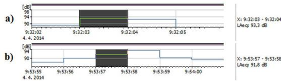
Fig. 9: Graph of the noise course at the cross sectional spruce wood cutting: feeding speed  $v_f = 12$  m·min<sup>-1</sup>, a) circular saw blade 1, b) circular saw blade 2.
