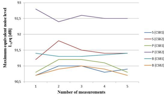
Fig. 8: Comparison of noise level at circular saw blades: feeding speed  $v_f = 4$  m·min<sup>-1</sup>, S (spruce), P (pine), B (beech), CSB1 – circular saw blade 1, CSB2 – circular saw blade 2.
