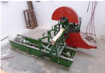
Fig. 1: Measuring equipment for cross-cutting wood.
