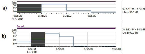
Fig. 11: Graph of the noise course at the cross sectional beech wood cutting: feeding speed  $v_f = 12 \text{ m}\cdot\text{min}^{-1}$ , a) circular saw blade 1, b) circular saw blade 2.
