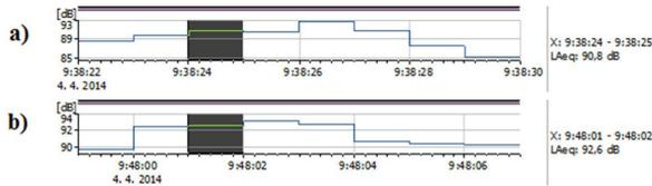
Fig. 6: Graph of the noise course in the cross sectional wood cutting: Feeding speed  $v_f = 4 \text{ m}\cdot\text{min}^{-1}$ , wood species (pine), a) circular saw blade 1, b) circular saw blade 2.
