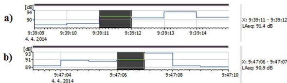
Fig. 7: Graph of the noise course in the cross sectional wood cutting: Feeding speed  $v_f = 4 \text{ m}\cdot\text{min}^{-1}$ , wood species (beech), a) circular saw blade 1, b) circular saw blade 2.
