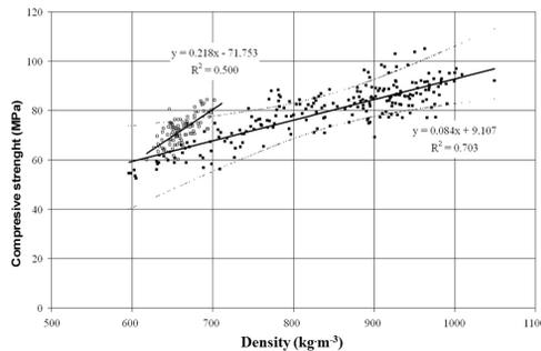
Fig. 4: Relationship between compressive strength along the fibres and the density of the timber in air-dry.
