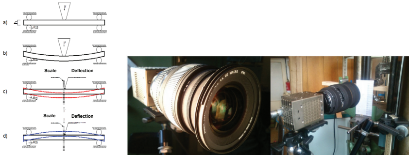
Fig. 1: Illustration of test of attenuation rate of deflection.
