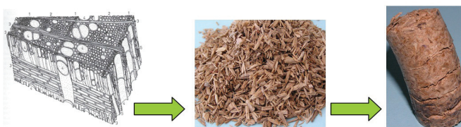
Fig. 3: Three-dimensional cross-section of hardwood – oak (left), oak wood sawdust (in the middle) prepared for pressing and pressed briquette from oak wood sawdust (right) (Požgaj et al. 1997, Križan and Svátek 2010).
