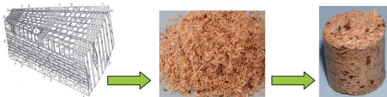
Fig. 2: Three-dimensional cross-section of softwood – pine wood (left), pine sawdust (in the middle) prepared for pressing and pressed briquette from pine wood sawdust (right) (Požgaj et al. 1997, Križan and Svátek 2010).
