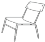
Fig. 1: Chair and armchair made of molded veneers. Fig. 2: Bending the veneer package in real process: 1 -upper mold; 2-veneer package; 3-lower mold.
