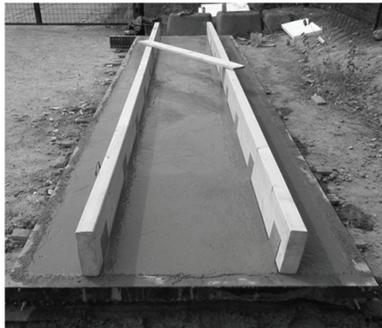
Fig. 3: Picture of timber-concrete composite panel (sample B).
