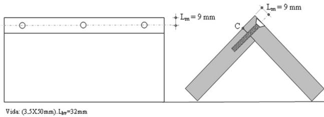
Fig. 5: Screw joint.
