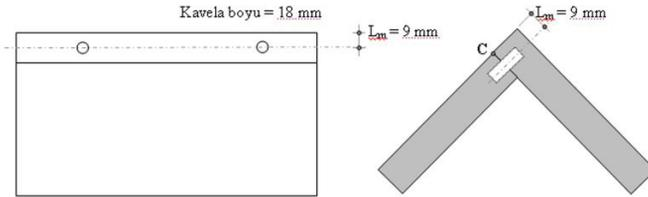
Fig. 3: Dowel joint.
