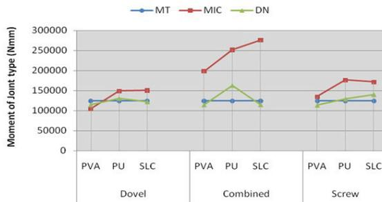
Fig. 7: Sufficiency of experimental joint moment to according theoretical earthquake moment.
