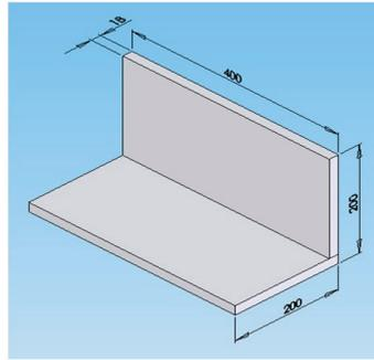
Fig. 6: Test sample (dimensions in mm).
