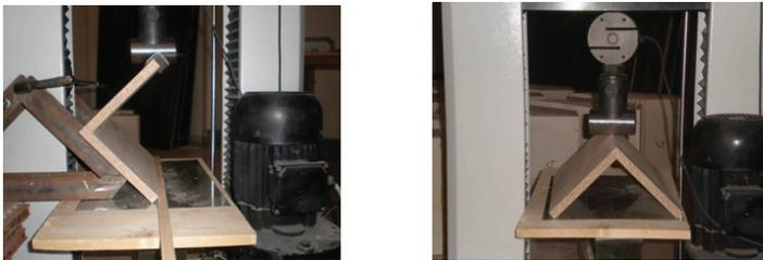
Fig. 8: Diagonal compression and tensile test.
