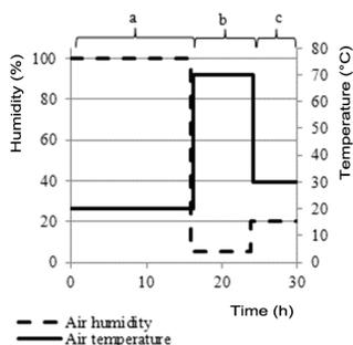
Fig. 2: Changes in humidity and temperature during full one cycle of weathering: a) soaking in water for 16 hours, b) drying at  $70^\circ \text{C}$  for 8 h, c) UV irradiation for 6 hours.
