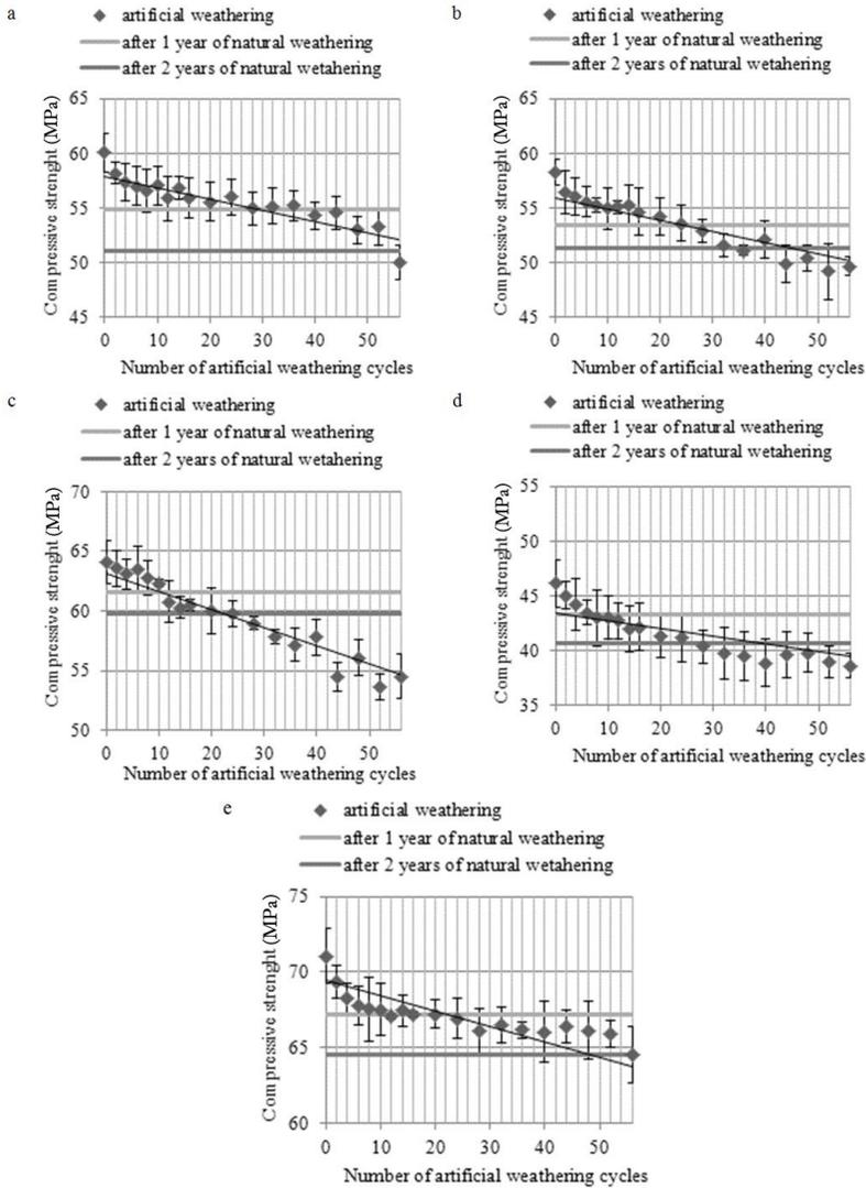
Fig. 1: Statement of results testing mechanical properties of wood during artificial and natural weathering: a) – heartwood of Scots pine, b) – sapwood of Scots pine, c) – garapa, d) – European oak, e) – angelim pedra.
